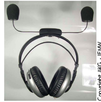
Figure 2 Tracking transmitter integrated on headset
