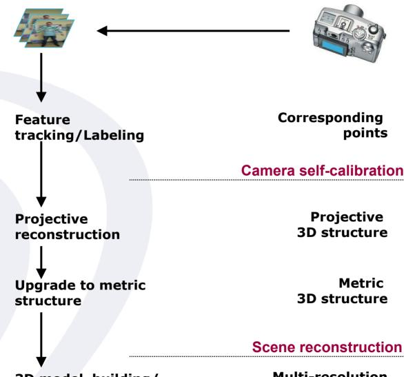
3D model building/ voxel carving Multi-resolution 3D voxel model •**Tracking** : the user identifies several relevant points in a reference image and tracks them throughout the sequence
